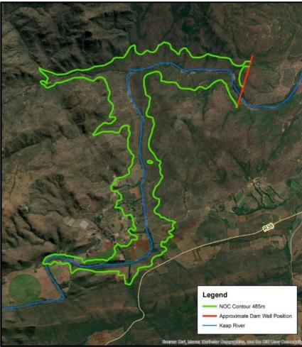
Water in the weir dams up within the river channel section for a distance of about 640 m where a very prominent granite rock outcrop forms an impressive continuous rock outcrop in the river section of approximately 250 m x 90 m, at the upstream end of the prominent gorge. Due to the presence of the weir and widespread water upstream of it, access for geophysical surveys and drilling operations is deemed very difficult.
