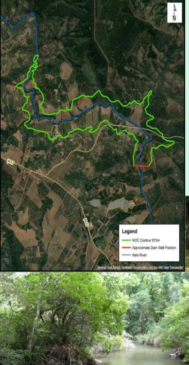
The site has an asymmetrical shape with a steeper right flank that is covered by scattered granite gneiss outcrop. A distinct north-south striking shear zone intersects the upper right flank. This feature is easily recognised by widespread pegmatite and vein quartz which also form somewhat of a ridge.
