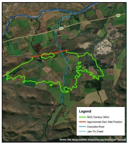
Strathmore Dam Site is an off-channel dam straddling two north-flowing streams. These are separated by a low hill which forms part of a distinct almost east-west striking low hill range. A third stream flows northwards along the far eastern portion of the reservoir (Salt Creek) which will also require a saddle dam pending the reservoir level. The entire reservoir area is under cultivation, mostly sugar cane.
