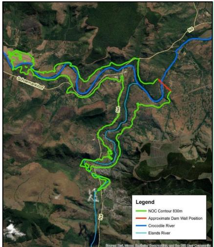
The Montrose dam site has an asymmetrical shape with the right flank significantly flatter than the left flank. Whilst vehicle access is possible from the right flank, the left flank access is difficult without any paths or tracks noticeable. It will be difficult to establish drilling equipment on the steep left flank. Widespread granite rock outcrops were however observed on the left flank.
